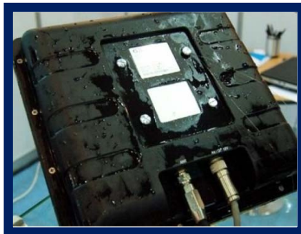
IP67 Underwater Immersion Test
