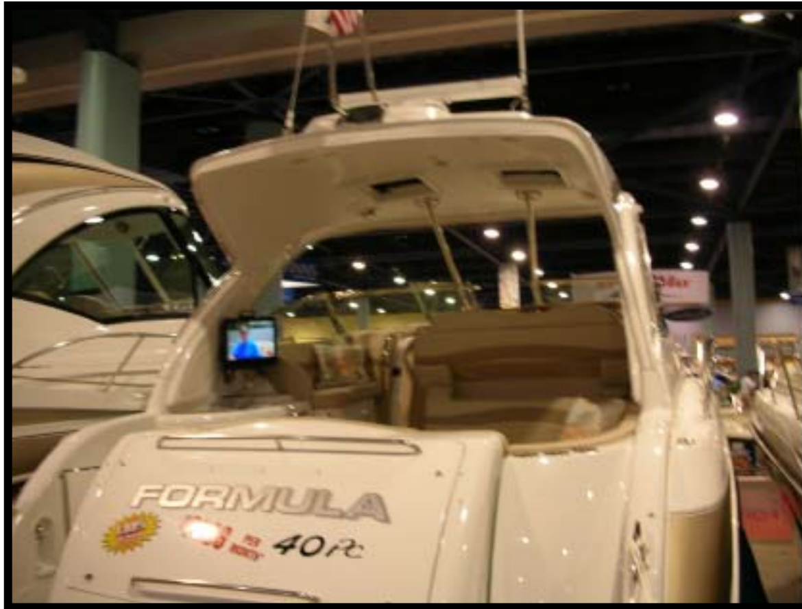
17" LCD TV mounted on a VESA 100mm Wall Mount Installed in a Formula 40C, Feb 2009
