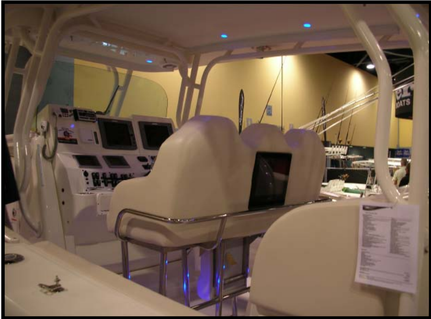
15" Waterproof Cockpit LCD (Side View) Installed on the Back Seat of a 41' Hydra-Sport in lean post, 2009
