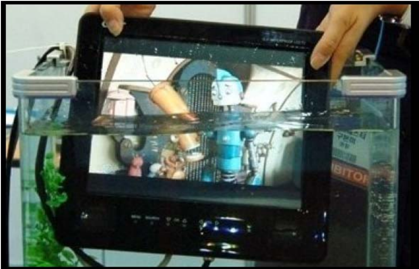
15" Waterproof LCD Waterproof Test in a Water Tank
