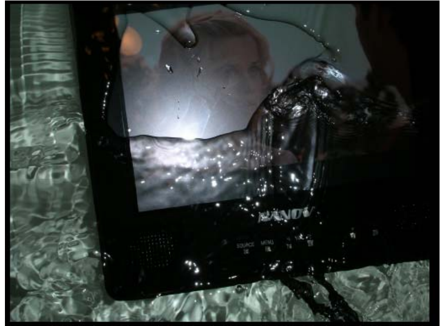
15" Waterproof LCD Completely Submerged in Water
