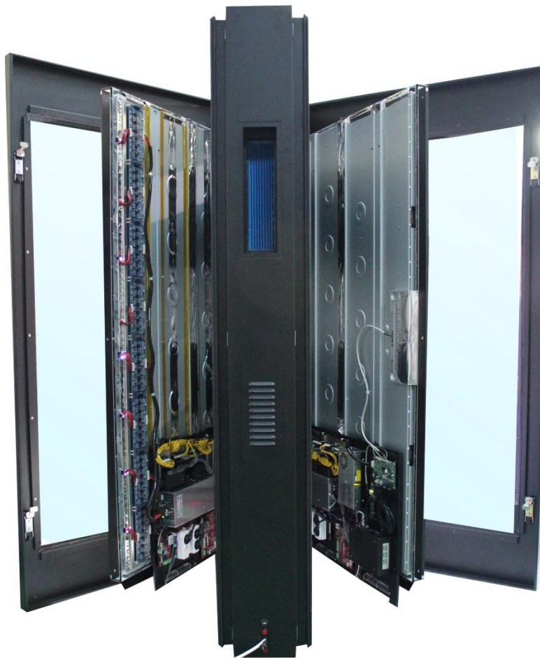
Door Opening Maintenance Concept
